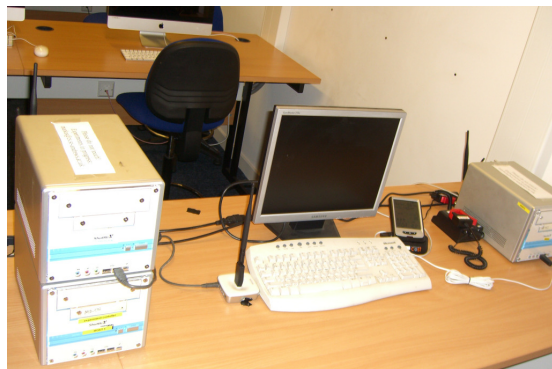
Fig. 3. Some nodes from our testbed. 1. The WiSpy DBx probe with antenna, mounted in a desktop USB hub. 2. The CC128 power meter and its power clamp (behind the CC128 LCD screen).
